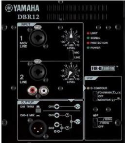
Connect the XLR plugs into both Yamaha DBR12 monitors to INPUT 1 (photo above).
