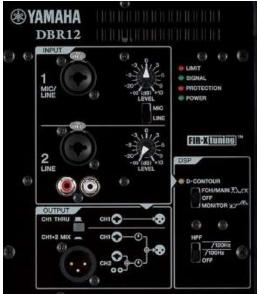
Connect the XLR plugs into both monitors to INPUT 1 (photo above).
