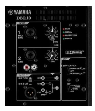
Connect the XLR plug to the floor monitor to INPUT 1 (photo above).
